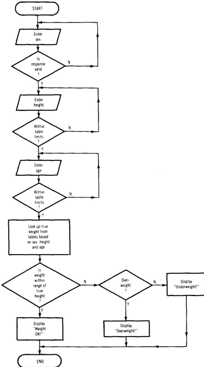
Fig. 3-1. Flowchart of the weight example program.
