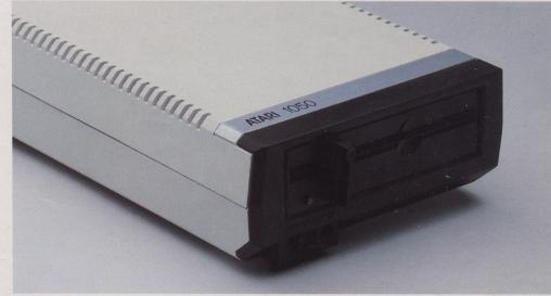
When you turn on the computer, DOS loads automatically. If you turn up the volume on your TV set while DOS is loading, you'll hear a series of beeps. This is perfectly normal and lets you know DOS is being loaded into the computer.
