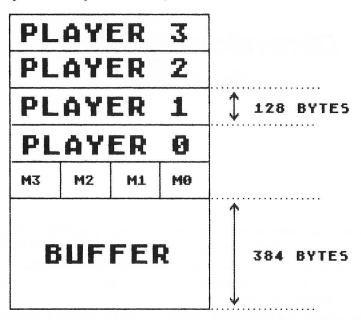
Note that this diagram shows the PM memory organization for what is called **double-line resolution**. Double-line resolution simply means that two lines are used to display each byte in PM memory. That is, if a bit is set to "1," then two pixels (one underneath the other) are lit up. We'll talk about double-line resolution in more detail later. Just remember that this diagram is for double-line resolution. Later we'll discuss single-line resolution (see Chapter 9).
