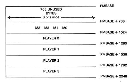
In single line resolution the television screen is divided vertically into 256 rows, so each of the above boxes represent 256 memory locations (bytes). The entire amount of memory the player-missile data base takes up is 1024 bytes in double line resolution and 2048 bytes in single line resolution. Since the data must be stored on a 1K or 2K boundary, we see that it exactly "fits" into a 1K or 2K section of memory.
