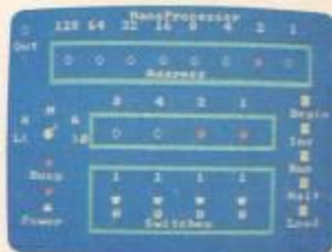
Photo 1: This shows the contents of the A register in the initial step of Sample Program 1. First, the program moves one number (3 or %0011) of an addition problem into A.
