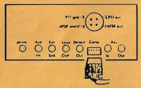
The computer cable is the only connection necessary between the computer and the Interface. Now follow the instructions in the Interface manual for connection of the Interface to the transceiver.
