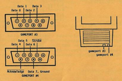
If your data lines are numbered one through eight instead of zero through seven use one as zero, two as one, three as two, and so on. Also use the signal ground, not the chasis ground.
