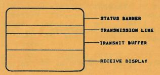
The lower portion of the screen will print the received signal while scrolling upward. The top portion of the screen is the status banner, showing the mode, speed, clock, and indicating transmit or receive.
