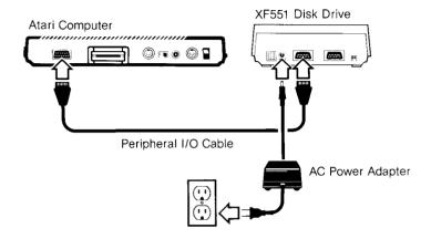
4. Plug one end of the peripheral I/O cable into the jack marked "Peripheral" on the back panel of the computer. Plug the other end of the cable into either of the two jacks marked "Peripheral" on the back of the disk drive.
