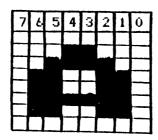
Therefore, to produce blue and gold objects, you only need to design your shape using either bits 7.5.3, and 1, or 6.4.2, and
