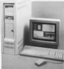
■ Atari's Transputer Workstation as demonstrated at the recent "What?" show. Full production should start in April. The graphics processor, called Helix, is capable of some stunning screen resolutions: 1280 by 800 using 18 colours from a palette of 4096, 1024 by 768 using 256 colours from a palette of 16 million, 640 by 480 using 256 colours from 65 million and 312 by 480 in True colour.
