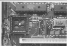
1. Remove the blitter socket with a solder sucker. Try not to suck near the circuit board at the same time. Remove the metal bar lying across the blitter socket. Use a clean烙铁.
