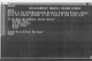
■ ANSI codes embedded within ECHO comments. Don't forget to put a ESC[0m code at the end to reset the text to normal.
