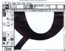
Fig. 3. Calamus outline fonts are scalable to 999.9 points on both the screen and printer in increments of 1/10th of a point.
