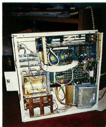
The Atari Transputer Workstation (ATW) has been engineered into a floor-standing tower design. It will enter production in early 1989.
