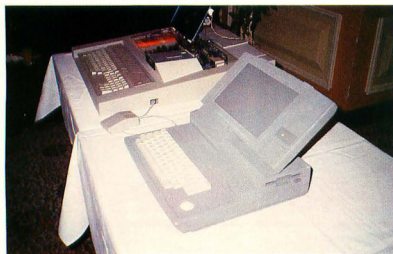
"I want one of those" was the most heard comment at Atari's developer's party. They were referring to the new ST laptop computer, shown here in both mock-up and engineering prototype form. A bright backlit supertwist LCD screen displays a full 640 X 480 monochrome compatible screen.
