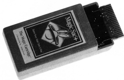
Data Pacific's Magic Sac is the first Macintosh emulator for the ST. It required 64K ROMs and therefore can't run programs requiring 128K ROMs.
