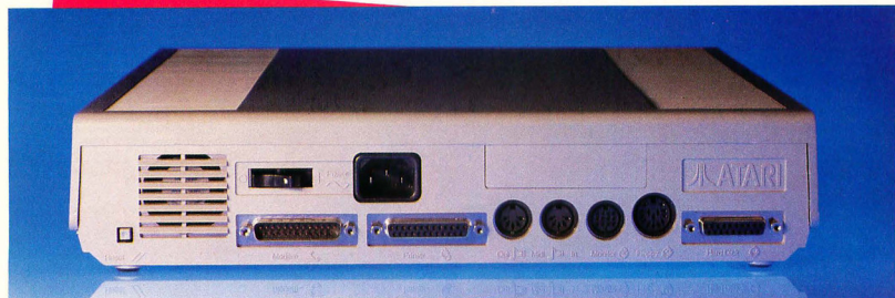
FIGURE 1. The back of the Mega. From left to right: the reset button, exhaust port for the internal fan, On/Off switch (top), modem port (below), power jack (top), printer port (below), expansion board cable access (top), MIDI Out, MIDI In, monitor port, floppy disk port, hard disk port.
