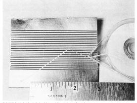
FIGURE 8: Unfinished, Etched Printed Circuit Board for Adapter.
