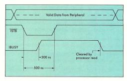
FIGURE 1: Typical 8255 Input Handshake Timing.
