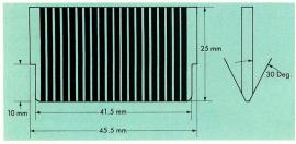
FIGURE 9: Finishing Dimensions for Adapter Card.
