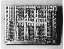
FIGURE 6: Photograph of Wiring Side of Interface.
