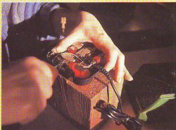
The micro switches are some of the few parts that are imported. Carefully positioned in the base, all the switches are thoroughly tested before the stick is passed.
