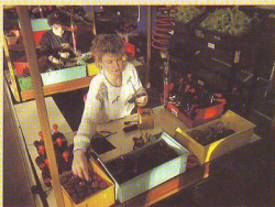
The skilled workers have all the components close at hand. The top section comes with the stick already in place. The buttons are the first parts to be added.
