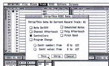
Breakthrough has a Thin/Strip MIDI Data function which can help ease controller overload problems.
