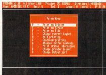
Top 4 & 5 to move between windows, F10 to return to DOS to exit
