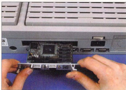
Fitting the Crazy Dots card into a Mega ST is extremely easy. Just open the VME access slot and push the card home. Crazy Dots is also available for the Mega ST
