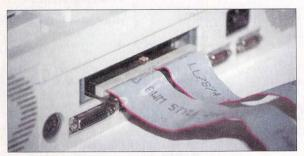
The Nova VME card is not screened, and a flimsy ribbon cable connects the VME interface to the rest of the hardware. Some extra electrical screening would be very helpful here
