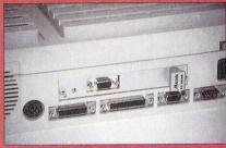
The Matrix card fits securely into the VME slot of a TT or Mega-STE
