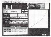
A fairly typical gradation or "gamma" curve to correct grey tone values - especially in mid-range - to compensate for the differences between monitor and print media
