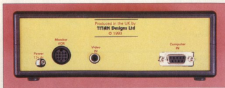
The back shows power, RGB output, video output and computer connections
