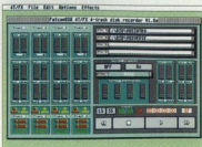
The 4T/FX program has only one window which is arranged like a four-track recorder. You can use it as four independent tracks or as two stereo pairs
