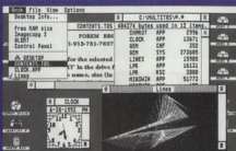
A TOS program called Contents is running in a background GEM window along with some other GEM programs
