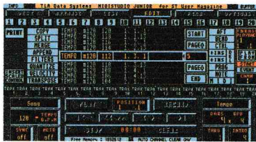
A dedicated tempo track showing a programmed rall from 120 to 60bpm across four bars
