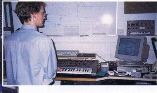
■ This is half of System Beat at the mixing desk. The ST controls all the juicy synths and drum machines, samplers and all the timing using C-Lab's Combiner, Untor and Steady Eye connected to the cartridge port.
