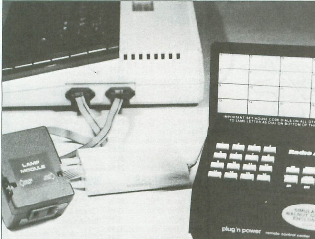
The X-10 interface connecting 800XL and X-10 controller. The lamp controller module is on the left.
