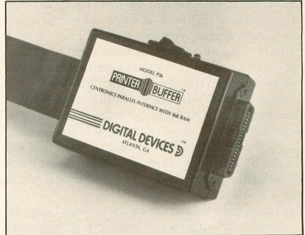
The *PRINTER BUFFER* works with any standard "Centronics" parallel computer or printer, including Digital Devices' *U-PRINT* printer interfaces for Apple, Atari, and Commodore computers. Available in 16K, 32K or 64K models, The *PRINTER BUFFER* is user-expandable in 16K increments. Perhaps best of all, the *PRINTER BUFFER* comes complete with all necessary cables, power supply, a comprehensive user's manual, a one-year limited warranty — and a price tag starting at \$119.95.
