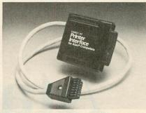
This unit negates the need for an Atari 850 interface module or special programming, and accepts all the standard Atari print commands. All cables and connectors are included, along with a lifetime warranty. \$79.95, CARDCO, Inc., 300 South Topeka, Wichita, KS 67202.
