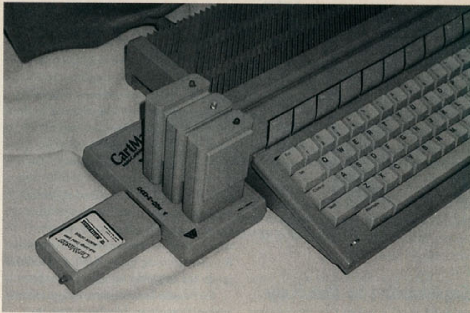
Cartmaster gives access to any one of up to four cartridges without manually switching them.
