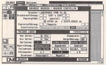
Preparing output of a single colour separation (Magenta) from Calamus SL to a Linotronic at the staggering resolution of 3387dpi.
